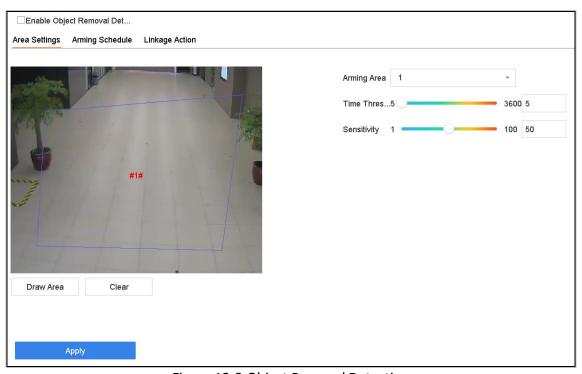
Figure 12-8 Object Removal Detection
