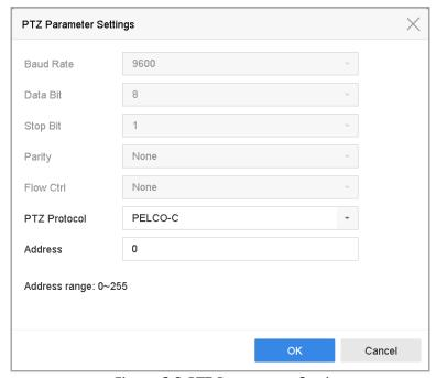
Figure 6-2 PTZ Parameters Settings
