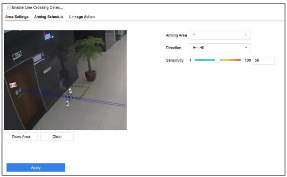
Figure 12-3 Line Crossing Detection
