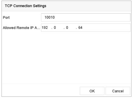
Figure 14-4 TCP Connection Settings
