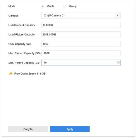
Figure 7-7 Storage Mode-HDD Quota
